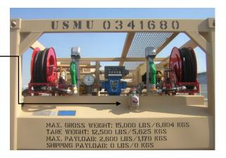
Two one inch by 50' hose reels for fueling two vehicles simultaneously.
