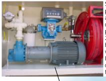
Sturdy cabinet protects pump, meter, filtration and hose reel from damage during transport and use. The 230/460 three-phase 3 horsepower pump provides receiving, recirculating, and dispensing capability at rates of 30 to 100 GPM.
